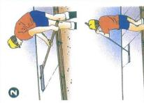
FLOATED FINISH (U2): Concrete surface handle lowered, on the returns stroke the being levelled with a "bull float". On the forward stroke the float is pushed with float is pulled with the handle raised.
